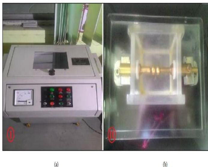
Fig. 4. 100kV BDV test Kit and Oil test cell
