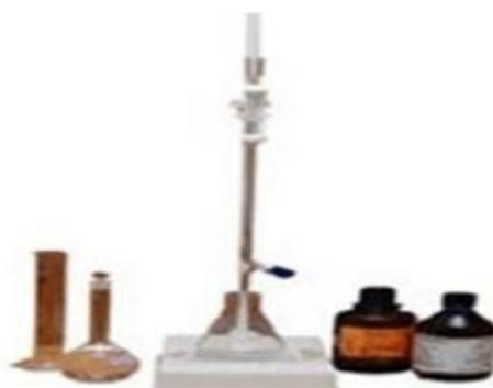
Fig.12. Image of Fire and Flash Point measurement setup
