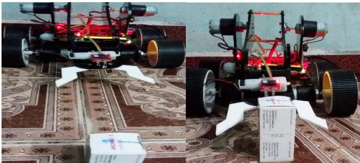
**Figure 9:** Placing the object by the robotic arm
