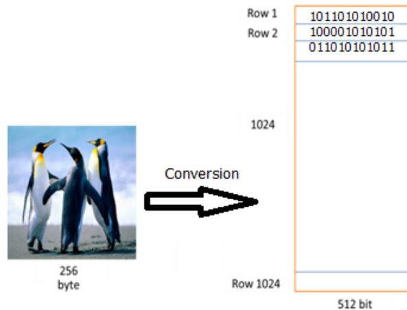
**Figure 3:** converting a sequential image to an array
