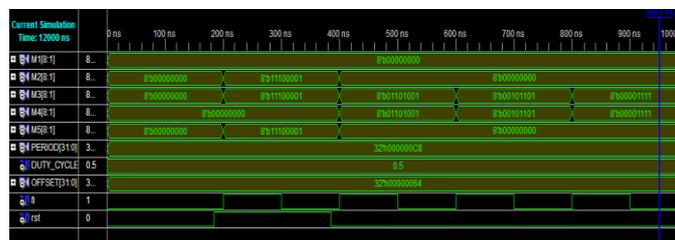
Fig 9. Testing of multiplier using the TPG produced by reconfigurable Johnson counter and LFSR
