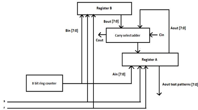
Fig 7. TPG using ring counter and Accumulator with CSA
