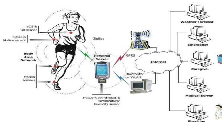
Figure 1: healthcare application using wireless sensor network
