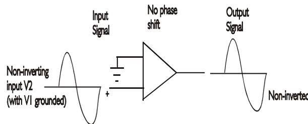
**Figure 5 Non-inverting mode of operational amplifier**
