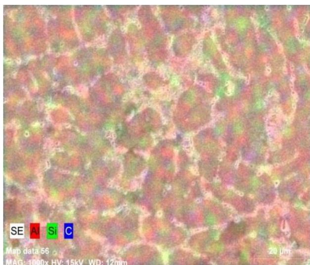
Figure 9 Colored SEM micrographs of Al/10wt%SiC
