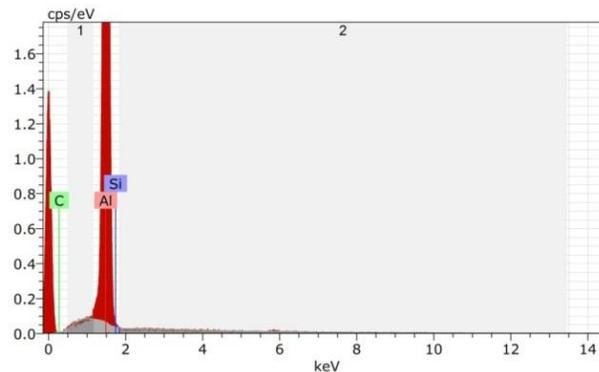
Figure 10 EDS spectra at the particle – matrix interface in Al/15wt SiC
