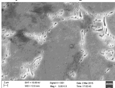
Fig 4 Sem image of Al/10wt%SiC
