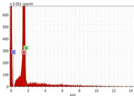
Figure 8 EDS spectra at the particle – matrix interface in Al/10wt SiC
