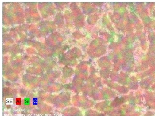
Figure 10 Colored SEM micrographs of Al/15wt%SiC
