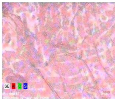
Figure 7 Colored SEM micrographs of Al/5wt% SiC
