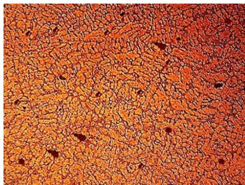
Figure 12 Phase segmentation of Al / 10 wt% SiC
