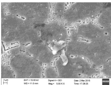
Fig 5 Sem image of Al/15wt%SiC
