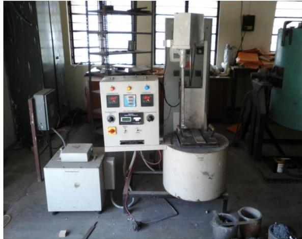
Fig 1 Stir casting furnace
