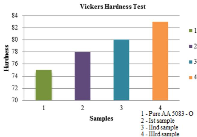
Figure 2 Vickers Hardness Test Result
