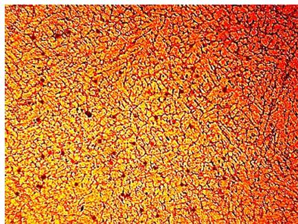
Figure 13 Phase segmentation of Al / 15 wt% SiC
