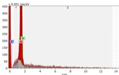
Figure 6 EDS spectra at the particle – matrix interface in Al/5wt% SiC
