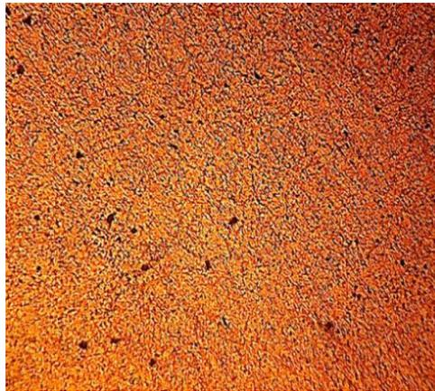
Figure 11 Phase segmentation of Al / 5 wt% SiC
