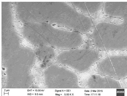
Fig 3 Sem image of Al/5wt%SiC
