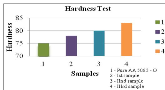
Fig 2 Vickers Hardness Test result
