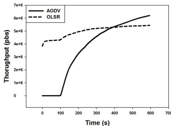
Figure 5: Throughput of (a) AODV, (b) OLSR protocols for video traffic
