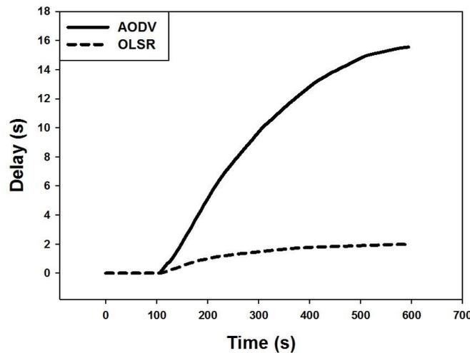
Figure 2: Average delay of (a) AODV, (b) OLSR protocols for video traffic
