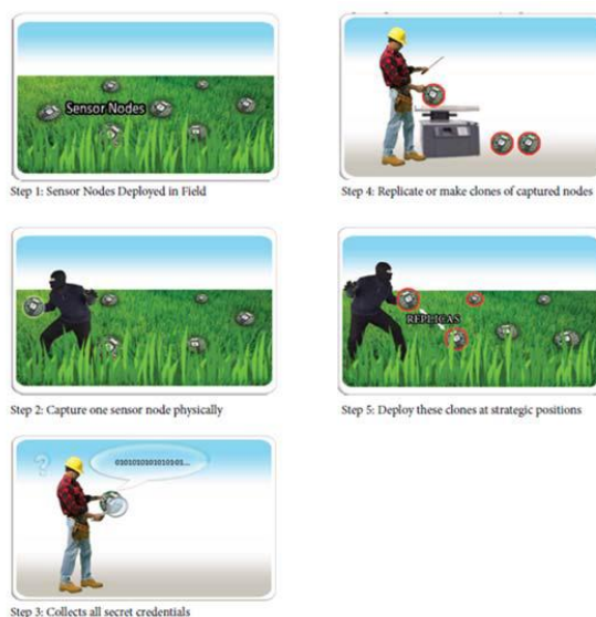
Figure 3:Steps of node replication attack
