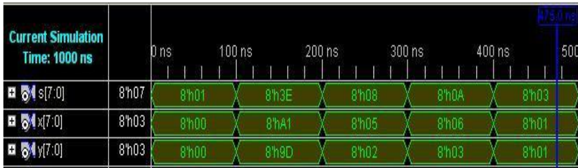
Simulation result of modulo 2^n+1 adder
