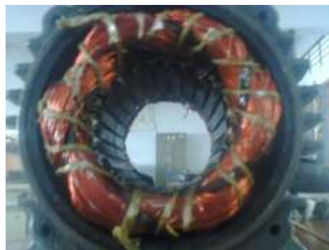
Figure 1 \text{Al}_2\text{O}_3 Nano Filler mixed Enamel coated Three phase induction motor
