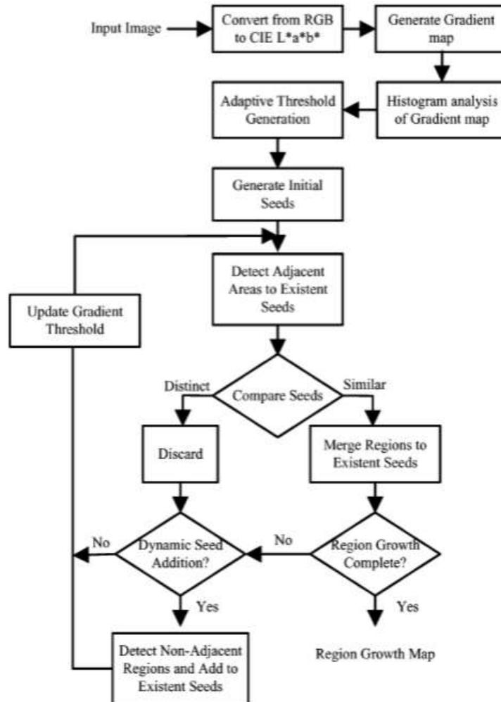
Figure 2: Flowchart of a region growth procedure
