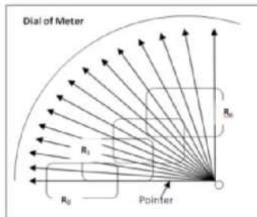
Figure 4: ROI Based Dynamic Sliding Window Technique
