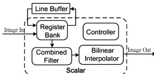
Figure 2 Block diagram of VLSI architecture
