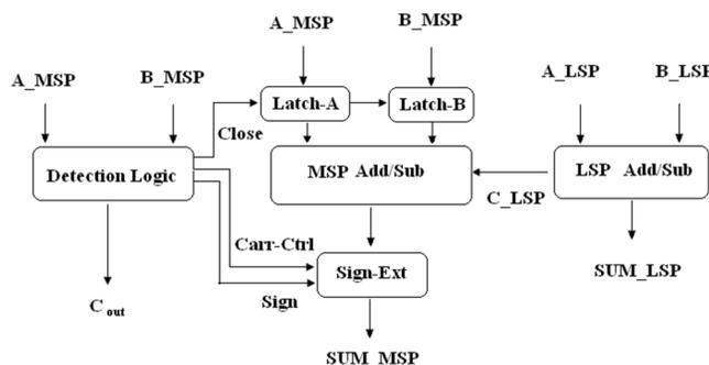
Figure 5 Block Diagram of SPST Technique
