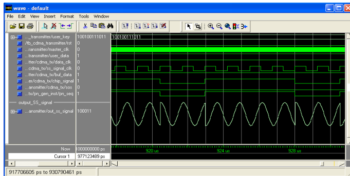
Figure 14 Simulation results for BPSK modulator
