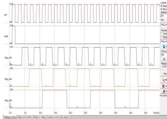
Fig.9- Simulation of Counter using .18 micron technology
