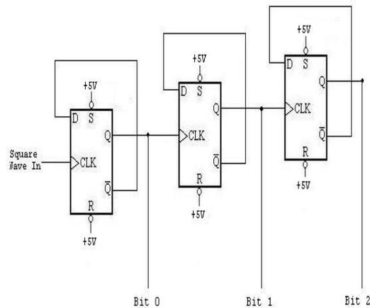
Fig.4 3 Bit Ripple Counter using D flip-flop
