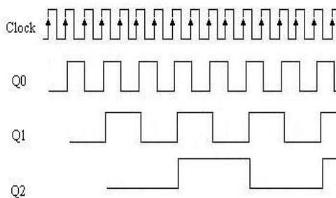
Fig.5 Timing Diagram of 3 Bit Ripple Counter
