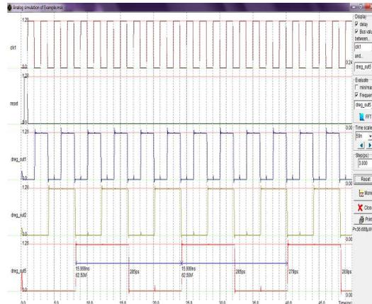
Fig.12- Simulation of Counter using 0.12 micron technology
