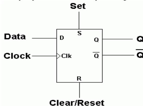
Fig.2 Symbol of D Flip-Flop
