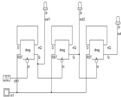
Fig.7 Design of 3 Bit Ripple Counter in DSCH2
