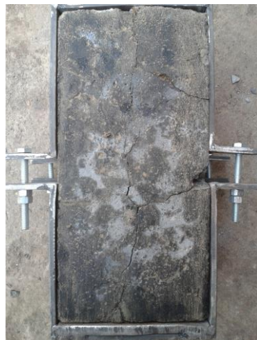
Initial failure mode Tension coupon test
