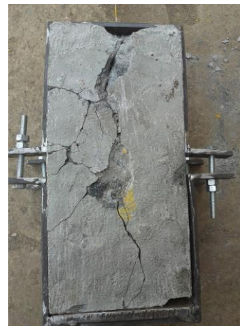
Initial failure mode Tension coupon test
