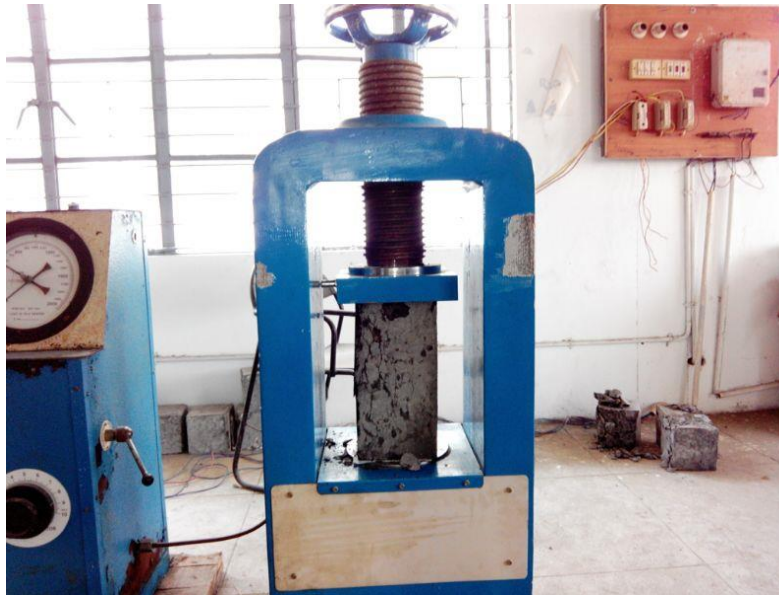
Failure of specimen
