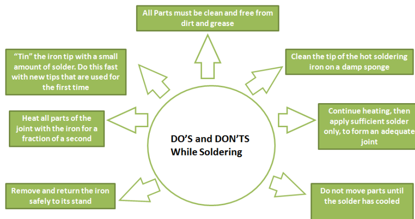
Figure 5 DO'S and DON'TS While Soldering
