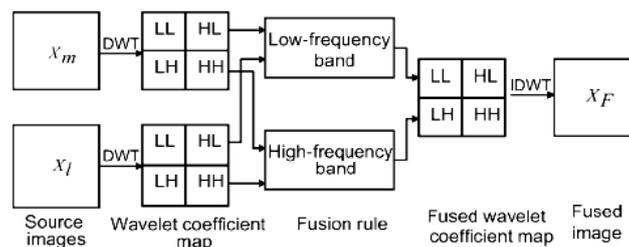
Figure 2. Process of image fusion based on the DWT
