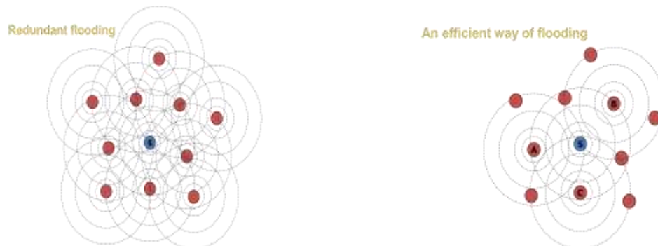
Fig 2.1 Efficient way of Flooding Scheme
