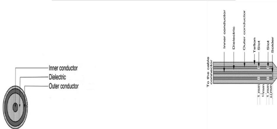
Figure1. Coaxial Antenna
