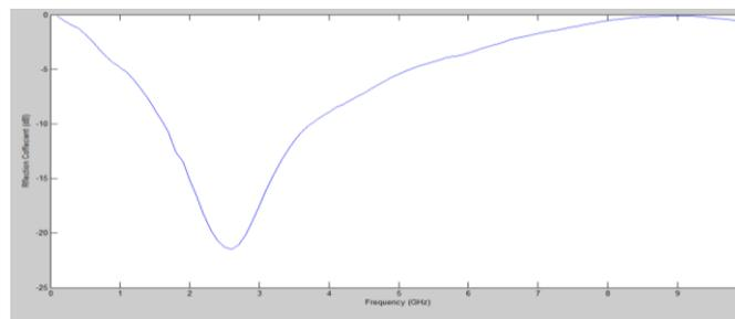
Figure 5 The simulated reflection coefficient expressed logarithmically
