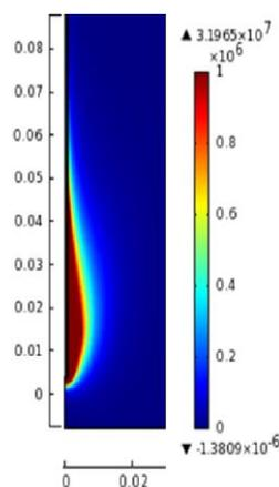
Figure 4 Surface: total power dissipation density(W/m<sup>3</sup>)
