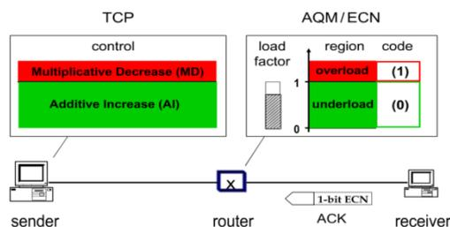
**Figure 6:** The TCP+AQM/ECN protocol congestion signal
